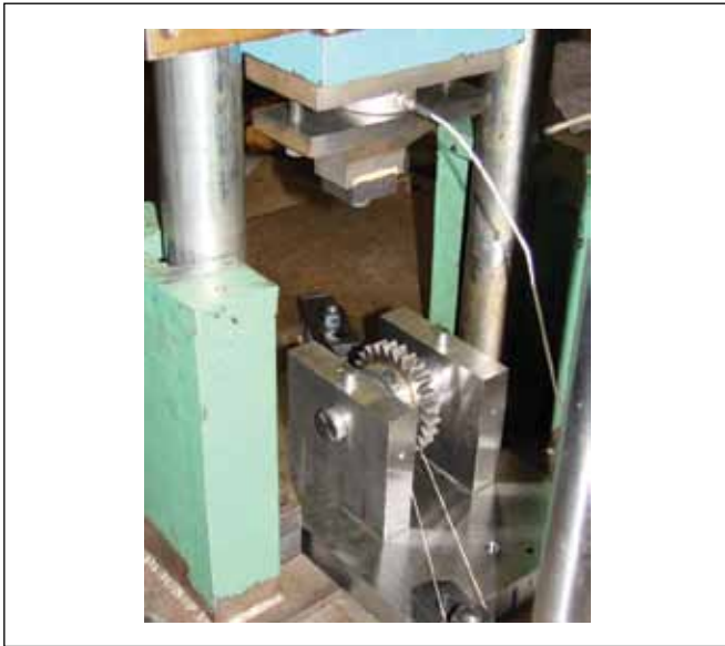
Figure 12—Tooth impact test machine.
