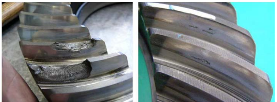
Figure 1 Flank breakage and pitting on wheel.
