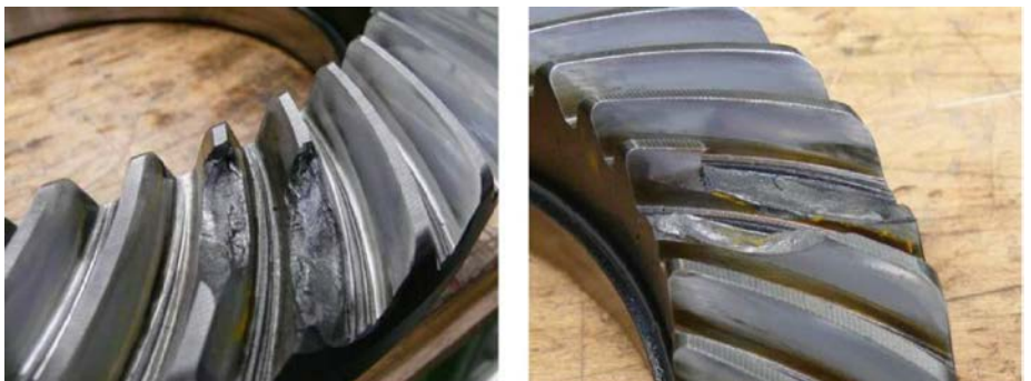
Figure 2 Flank breakage—two different wheels.
