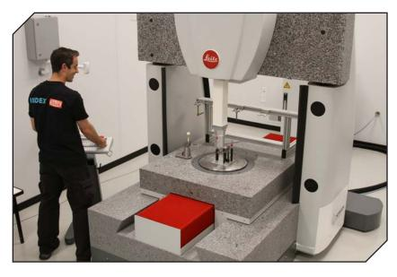
Index has already used the Leitz machine to good effect in proving its machining processes produce parts that meet the quality specifications of its customers.
