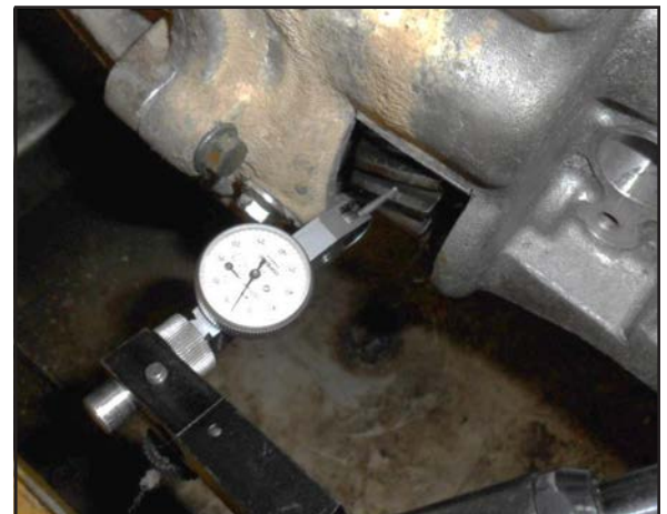
Figure 4 Backlash measurement of reverse idler gear.
