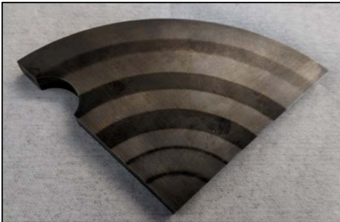
Figure 5 The standard sample as it appears after a good acid etch.
