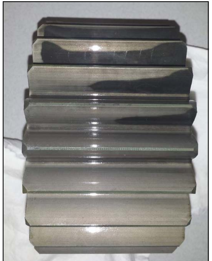
Figure 2 Example of burned gear after going through the acid etch series of tanks; dark areas show “temper-back,” with some visible cracking.
