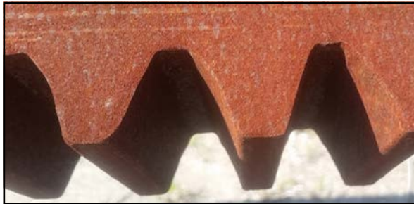
Figure 19 Rack removed from hull.
