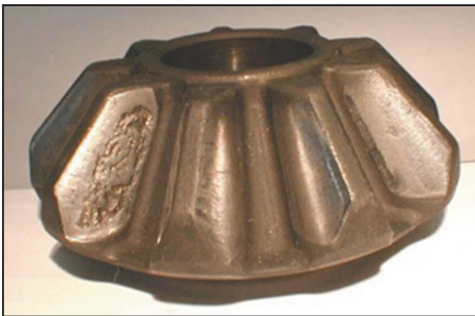
Figure 3 Forged differential gear with pittings.
