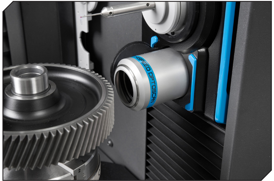
Pitch measurement with HISPEED OPTOSCAN.
