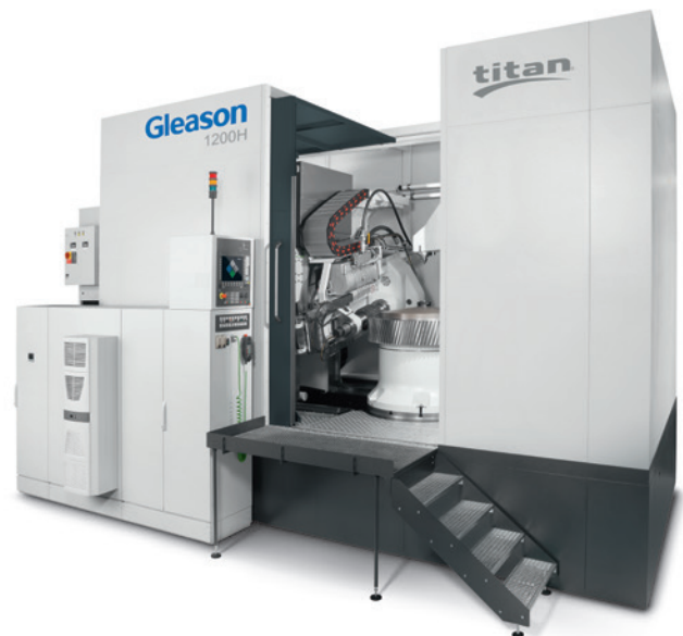
Figure 5 Gleason’s Titan 1200H has a tool changer that allows greater versatility.
