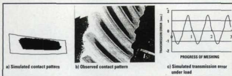
Figure 11—Loaded contact pattern on ring gear flank and the transmission error (input torque = 30 N-m).
