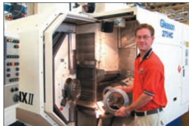
Figure 29—Real-life cutting machine based on a monolithic design.
