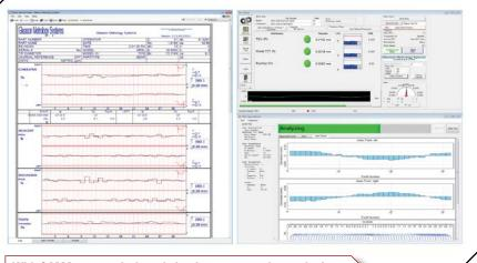
With GAMA gear analysis and charting output, options exist for AGMA, DIN, ISO as well as OEM specific analysis for the involute and index measurements, with common charting as seen on the popular GMS series of analytical machines.
