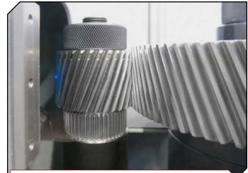
Non-contact (laser) index and profile inspection can be performed on all the gear teeth in a matter of just 10 to 15 seconds, as compared to several minutes when done conventionally.
