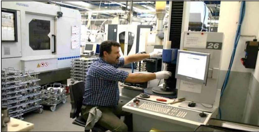
Figure 9 Gear measuring machines have for years been used directly in the production area. By adapting the roughness sensor on these machines, this is now also practiced for roughness measurement.
