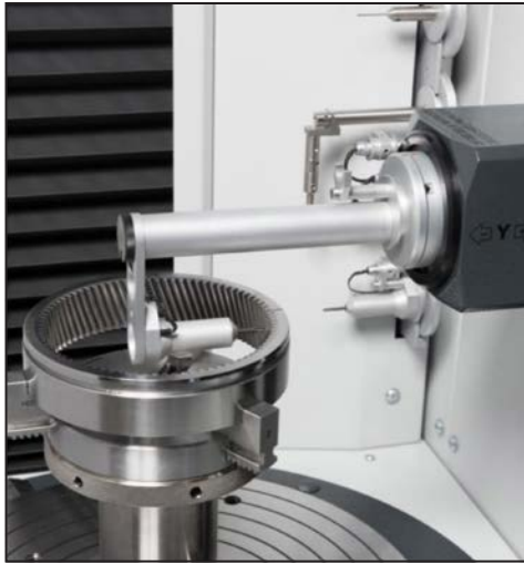
Figures 21 and 22 Roughness measurement of internal gears.
