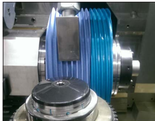
Figure 1 Polish-grinding with a combined grinding-polishing worm.
