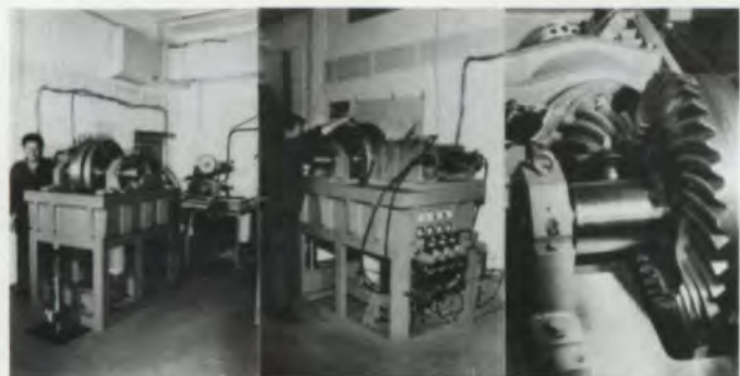
Fig. 6—Loading device for determination of tooth root stresses at bevel gears.
