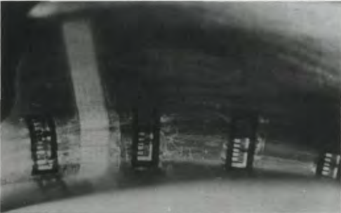
Fig. 2—Pinion tooth with 10-element strip gages (before they were wired).
