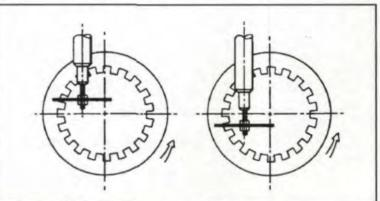
Fig. 11 - Setup for deburring square slots or splines.
