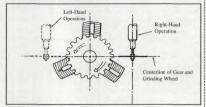
Fig. 5 - Aligning the grinding wheel to the center of the gear.
