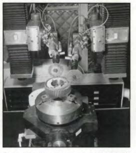
Fig. 2 — Deburring a spur gear with a brush followed by a grinding wheel.
