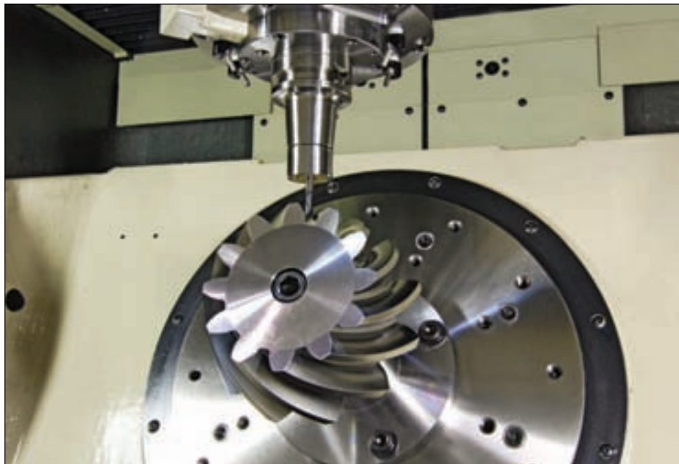
The Vertex five-axis machine cuts spiral gears up to 16 inches.
