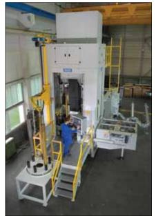
Advanced automation, material handling and CNC controls represent the latest in broaching technology. Pictured here is a 50-ton, two-station CNC helical broaching machine from Forst.
