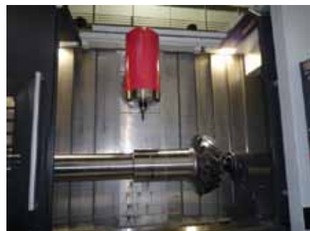
Figure 8—Pinion workpiece on multi-tasking machine.
