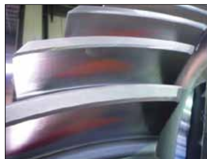
Figure 12—Tooth contact pattern of coast side.
