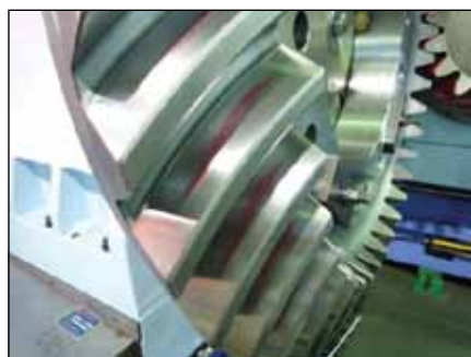
Figure 11—Tooth contact pattern of drive side.
