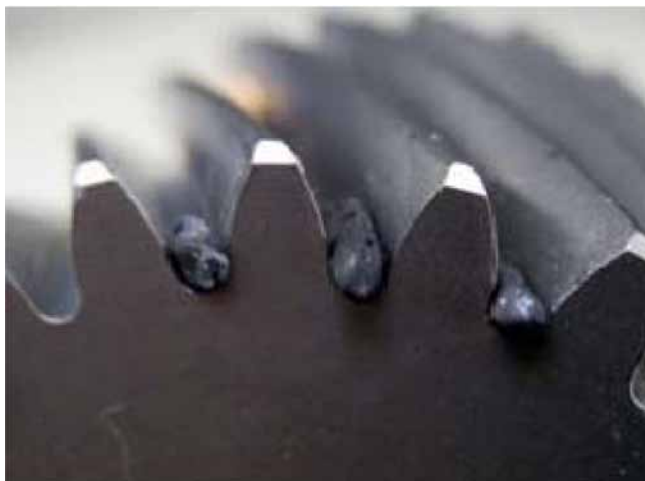
Figure 28—Gear B with smaller ISF media.
