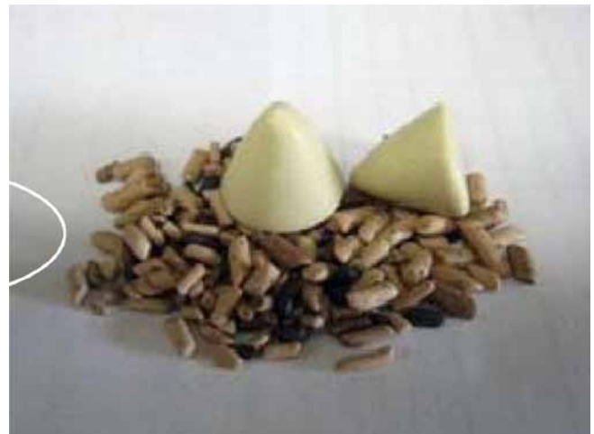
Figure 29—ISF process development: final ISF media mixture used for test gears.
