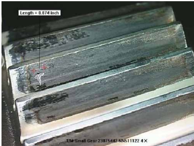
Figure 6—Baseline Gear C, Mesh 2: post-150-hour test.
