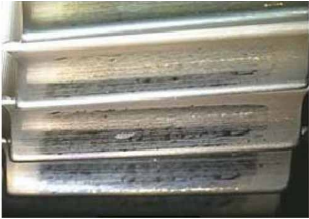
Figure 4—Baseline Gear A, Mesh 1, drive side: post-150-hour test.
