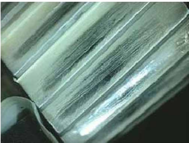
Figure 19—ISF Gear C, Mesh 2: post-150-hour test.
