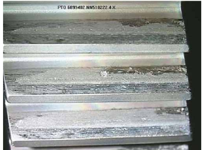
Figure 7—Baseline gear D, Mesh 2: post 150-hour test.
