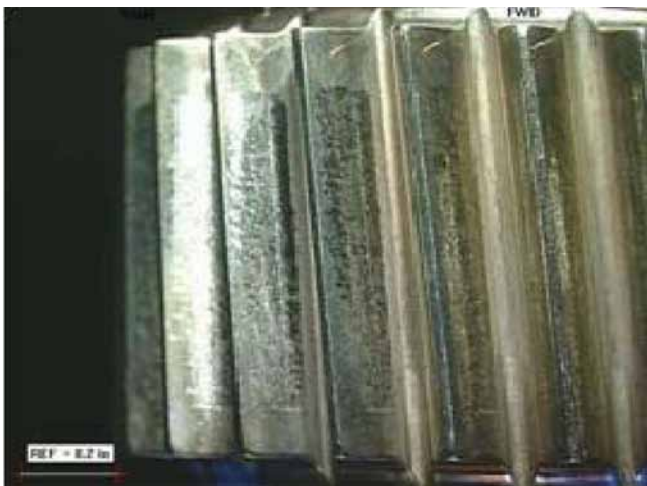
Figure 21—ISF Gear A, Mesh 1: post-2,000-hour test.
