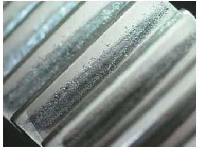
Figure 18—ISF Gear B, Mesh 1: post-150-hour test.
