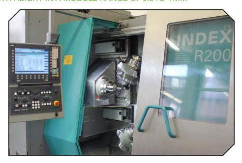
In addition to bar stock machining, which is best primarily for small quantities, for series production the R machine can be used as a pure gear cutting machine, working on the main and counter spindles simultaneously.
