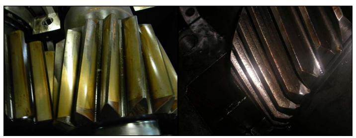
Pictured: one gear that has suffered light wear and can be reground (left) and a gear that will need to be replaced (right).
