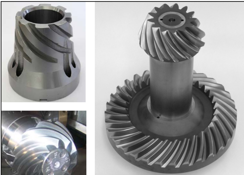
Figure 15 Different gear types machined with the UNIMILL process.
