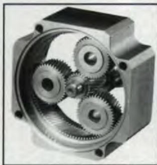
Fig. 3—In Bayside Control Group's precision gear set, even a film of lubricant can potentially be thick enough to cause a positioning error. A very light thixotropic grease not only passed rigorous life tests, it also lowered internal temperatures by five degrees.
