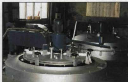
Figure 1—Conventional gas-carburizing furnaces. Maximum measurements of a gear can be 1.3 m in diameter, 2 m in height and 5,000 kg in weight. Carrier gas is endogas, enriching gas is propane.
