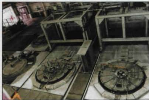
Figure 2—New gas-carburizing furnaces. Maximum measurements of a gear can be 2.5 m in diameter, 2.5 m in height, and 15,000 kg in weight. Carrier gas is a mixture of methanol and nitrogen, enriching gas is propane.
