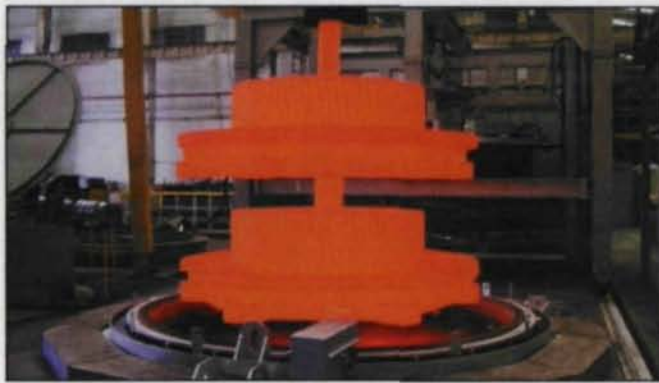
Figure 11—Just carburized gears are removed from a new furnace before quenching. Each gear has 78 teeth, each one 407 mm long, a module of 20, an outside diameter of 1,638 mm and is made of SCM420H, a JIS material specification. Hardness of carburized teeth is HRC 58–60, case depth is 5.5 mm.
