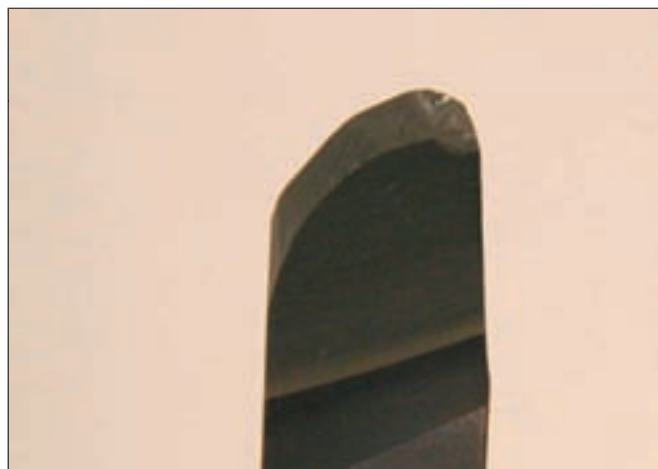
Figure 11—Large blade top chipping called “banana peel.”
