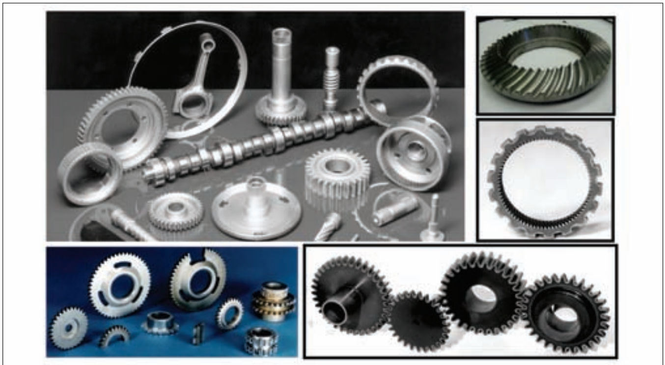
Figure 1—Typical induction hardened gears and critical components.
