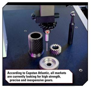
nificantly over the years, whether it be through the use of chrome-steel alloys, single press high dense technologies, or tooth flank densification to minimize contact fatigue issues (fretting). Bending fatigue strength has improved dramatically by achieving high (>7.4 g/cm³) core density with high tonnage part compaction, and minimum levels of organics (powder lubricants, etc..) in the raw material," Slattery said.
