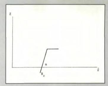
Fig. 6-Straight-Line Tooth Profile in the Normal Plane
