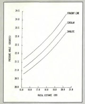
Fig. 9-Pressure Angle Variation for Three Cutter Profiles
