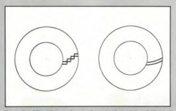
Fig. 2-Spiral Bevel Gear as a Limiting Form of a "Stepped" Straight-Toothed Gear
