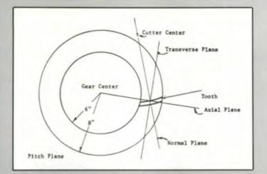
Fig. 1-Spiral Bevel Crown Gear and Identifying Planes
