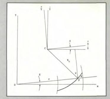
Fig. 4-Coordinate Geometry for a Typical Point P on the Tooth Centerline
