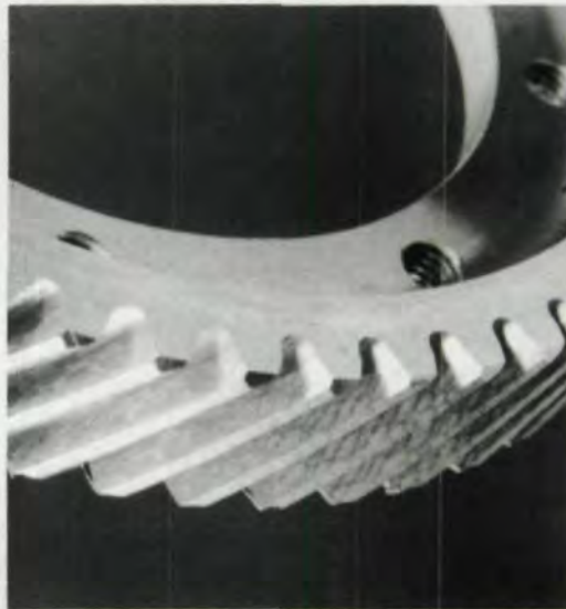
Fig. 2 - Gear tooth flanks produced by high feed rate, multi-thread hobbing.
