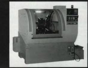
Introducing KOEPFER's newest machine: the MZ120. This machine is designed for fine pitch worm milling and hobbing applications. The MZ120 is a full CNC machine controlled by GE Fanuc. In line with KOEPFER tradition, the MZ120 can be equipped with a variety of flexible automation systems.
