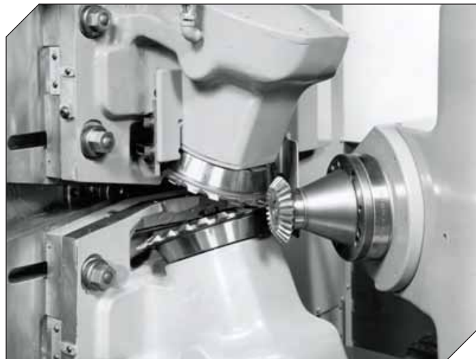
Figure 4 Coniflex cutting with interlocking HSS cutter disks.
