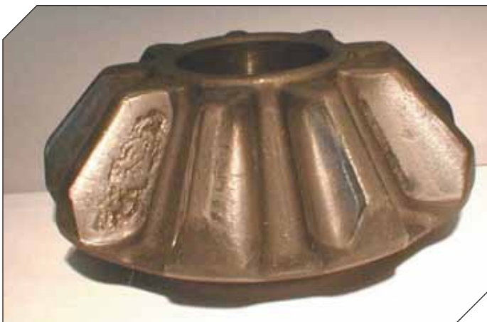
Figure 3 Forged differential gear with pitting.
