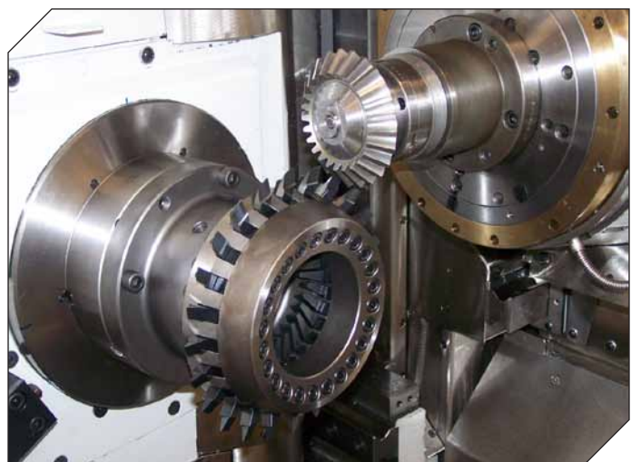
Figure 5 ConiflexPlus high speed dry cutting on a Phoenix 275HC machine.
