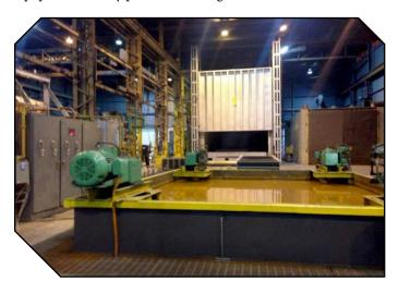
All equipment from both companies has been consolidated at the 65,000 square foot Complete facility in Milwaukee, where the highlight is a gas-fired car bottom furnace with a 53'×22'×14' workspace, powered by 40,000,000 BTUs with a 1,000,000-pound load capacity and operating temperatures to 2,150°F max.
