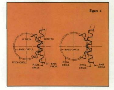
12-tooth pinion shown to the right of the diagram exhibits a much stronger tooth form as a result of 'addendum modification'. If the generating process is used to produce gears developed from the basic rack, the foregoing principles are fully exploited and the same cutter may be used to cut all numbers of teeth.
