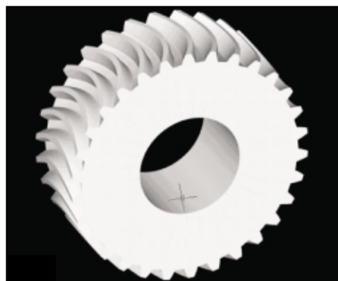
Figure 8—Pictorial representation of the curved face width spur gear, with modified geometry.
