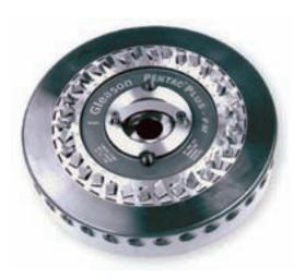
The Pentac Plus is the latest generation of Gleason's Pentac bevel gear cutting system. It is designed to allow much higher tool life and improved productivity, especially for cutters using multiple face blade geometry.
