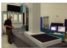
The LHGT 2600 Hybrid CMM and GMM is designed for wind energy industry measurement needs.
