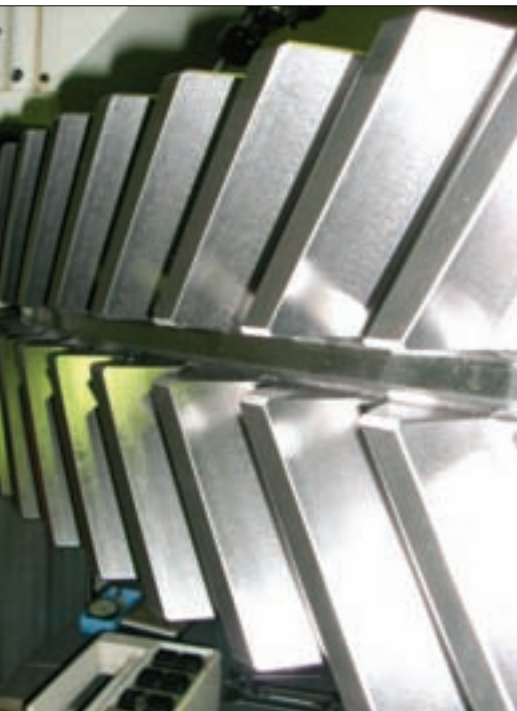
A coarse pitch double helical gear completely machined by Depo, including chamfering and deburring (courtesy of Depo).
