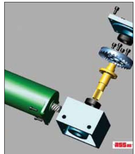
Figure 5—Automatic door moving system with Cylkro transmission.
