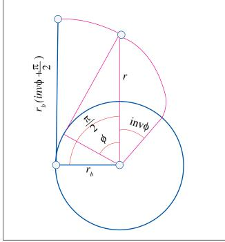
Figure 2—Transverse section of an involute worm.
