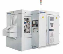
The Raso 200 Dynamic has been developed to offer all the characteristics of a gear shaving machine with a competitive price. With a footprint of just 4.4 square meters, it's also the most compact machine of the Sicmat Raso range. The Dynamic is the first shaving machine in the Raso family to utilize Siemens CNC Sinumerik 828D.
