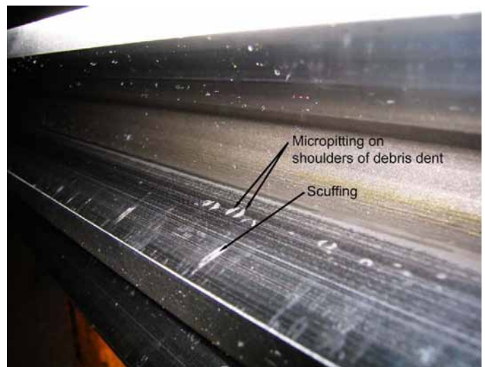
Figure 11 Wind turbine sun pinion with micropitting on shoulders of debris dents.
