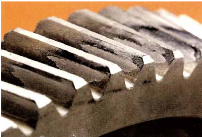
Figure 9 Micropitting pattern on a helical wheel that had some misalignment (courtesy of Caterpillar).
