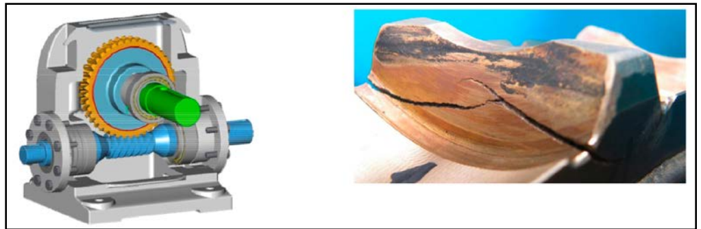
Figure 1 (Left): CAD model of the worm gear set; right: tooth with cracks at the tooth root notch.
