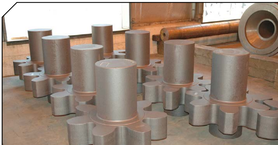
An integrally forged shaft, made as a tooled double hub, then torch cut and finished. The part displays a number of different process including loose tooling, torch cutting, heat treating and machining (courtesy of Scot Forge).
