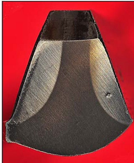
Figure 1 Bending fatigue failure of induction-hardened gear.
