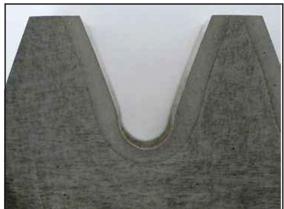
Figure 4b Induction hardening with cooling jets turned on (Ref. 3).
