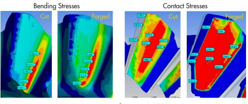
Torque on one side gear = 1,000 Nm Figure 2—Stress comparison, Coniflex Pro cut versus forged (input torque = 1,000 Nm).
