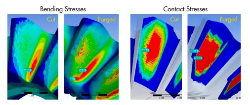
Torque on one side gear = 200 Nm Figure 1—Stress comparison, Coniflex Pro cut vs. forged (input torque = 200 Nm).
