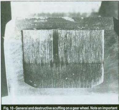
wear of the profile with the presence of radial rough irregular streaks. Also note a metal pull-off toward the tip of the tooth.
