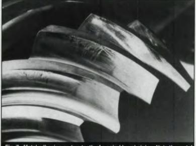
Fig. 7 - Metal adhesion on two teeth of a spiral bevel pinion. Note the metal pull-off located on the contact surface and in the maximum slipping zone with transverse scratches in the direction of the sliding motion.
