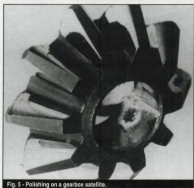
wear does not cause large variations in the shape and in the dimensions of gear teeth. However, when examined under a microscope, the structure just below the contact surface reveals the presence of plastic flows in the material under slippage. Sometimes very localized overheating traces near the surface are also encountered. The polishing encourages establishing gear teeth contact patterns in service and allows obtaining a good conformity of surfaces in contact.
