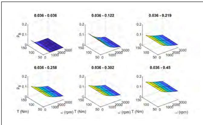
Figure 7—Boundary area contact ratio for 0036 surface pairings.
