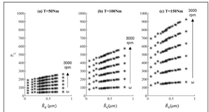
Figure 8—Predicted power loss vs. composite roughness.
