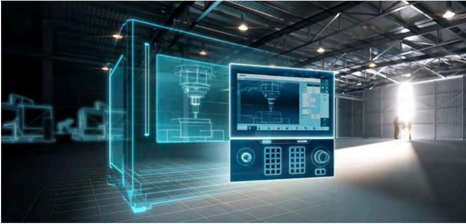
for builders and users alike. Machine concepts and functions can be discussed and planned even before real hardware is available. Realistic simulation enables CNC machine users to simulate the programming of workpieces and the setup and operation of machine tools completely on the PC. Even training can be carried out using the digital twin instead of training on the actual machine.
