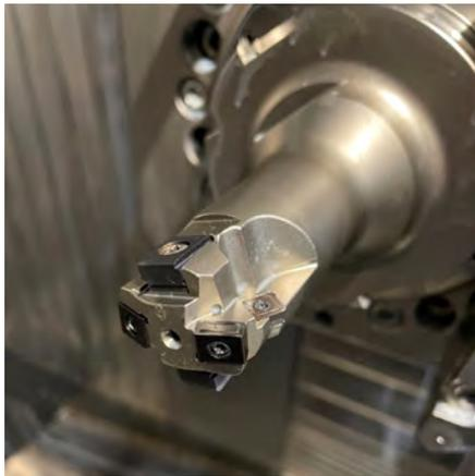
allows for higher feed speeds while at the same time producing a better surface quality. Plus, the new inserts provide a much longer tool life as compared to their predecessors.
