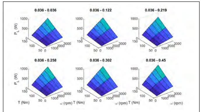
Figure 5—Predicted mechanical power loss for 0036 surface pairings.
