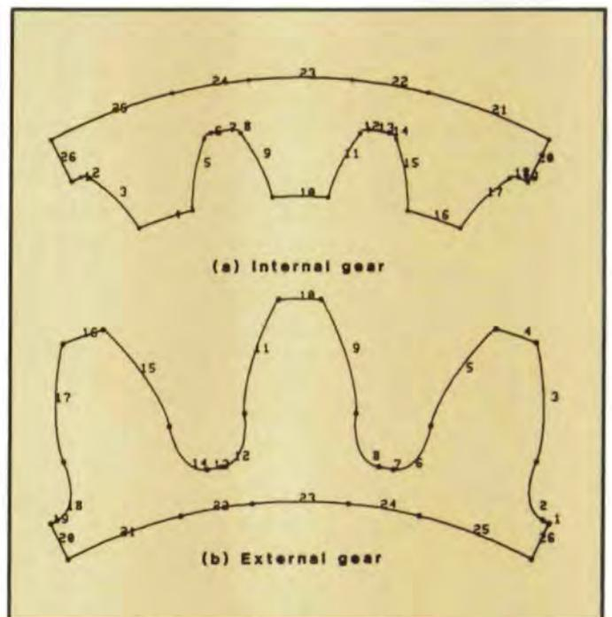
Fig. 2—Gear tooth boundary and its subdivision into segments.
