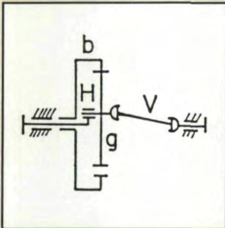
Fig. 1 - KHV gearing.
