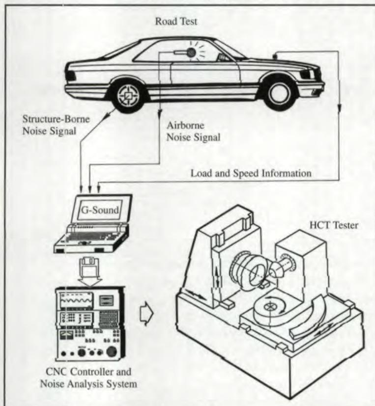
Fig. 6 — Closed loop between vehicle and HCT tester.
