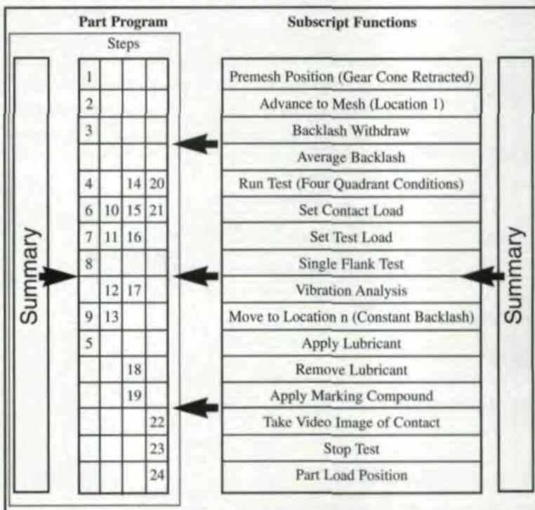
Fig. 5 — Modular structure of HCT tester operation software.
