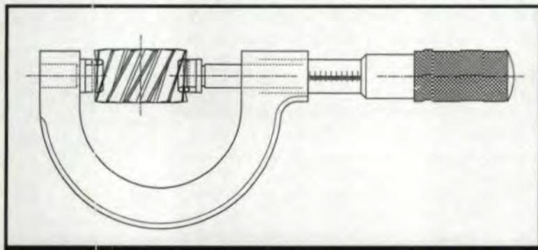
Fig. 1 — Orientation of gear and pin anvils.
