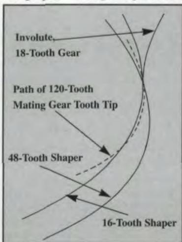
Fig. 2 — Fillets generated by different sized shapers.
