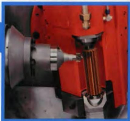
■ **Designed for dry.** The Pfauter P100 is a true dry carbide hobbing machine. The horizontal work spindle facilitates chip removal; and a work area completely enclosed in a stainless steel shroud directs chips downward and completely away from the work area. There's simply no place for "hot" chips to accumulate in a dry operation—the P100 is thermally stable!
