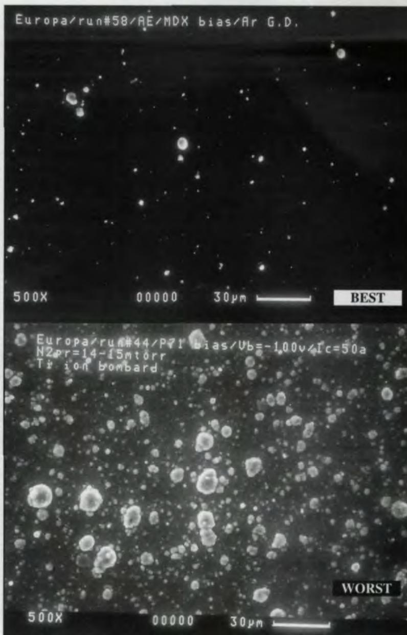
Fig. 4 — SEM photomicrographs of TiN surface for the different bias power supplies.
