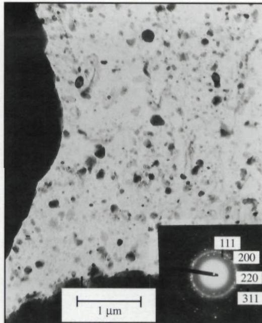
Fig. 4c — Microcarbides (Mo<sub>2</sub>C) precipitated by ausrolling.
