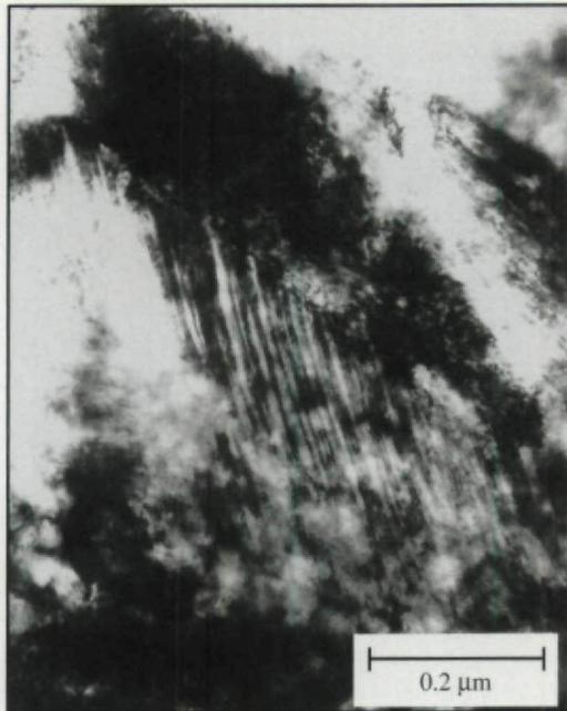
Fig. 4a — Ausrolled microtwins.
