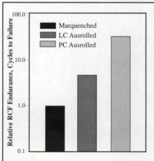
Fig. 6 — Relative rolling fatigue endurance and processing.
